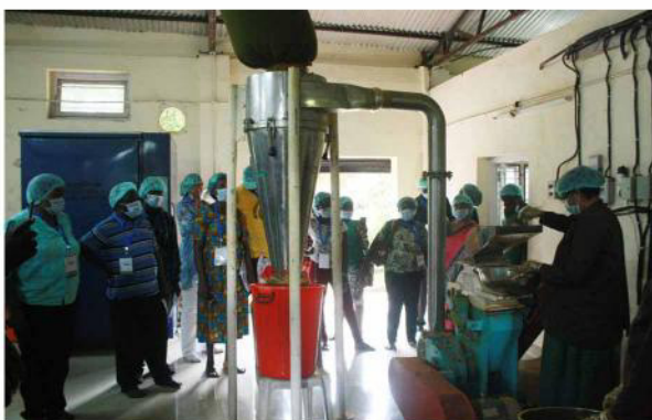
Demonstration of pulverizing unit
