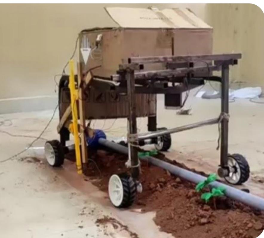
Once placed in the field rows, the bot automatically moves forward & backward in the field inserting sensors randomly in half of the field. The sensors inserted in the field provides the Bot with data which is analysed for different parameters like soil moisture, temperature, humidity, pH levels etc. Based on the analysis the soil requirement is assessed and instruction will be sent to the pump directly without requiring any human intervention.
