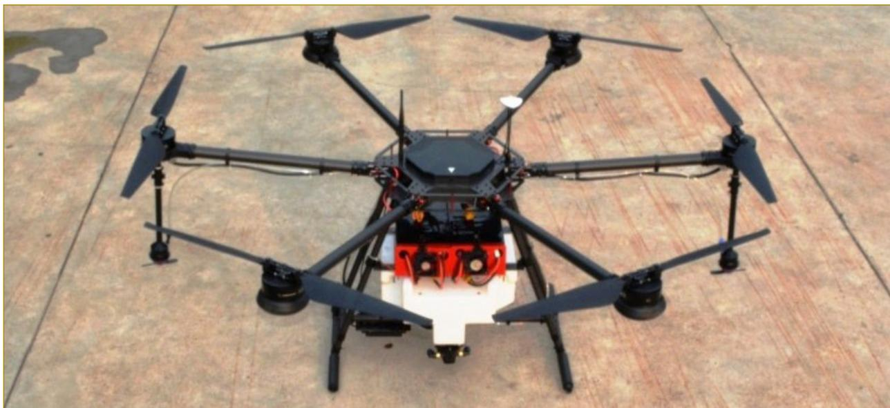
**Thanos's In-house built Spraying Drone**
