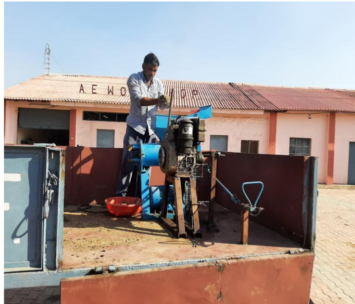
Fig. 4 Feed pellet formation with portable feed pellet making machine
