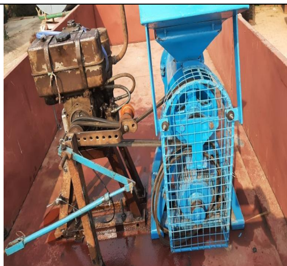
Fig. 3 Power transmission system of portable feed pellet making machine
