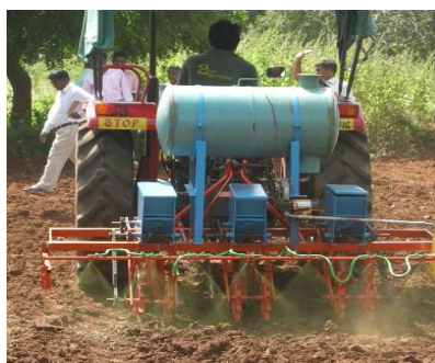
Figure 7.6: Precision Planter cum herbicide applicator
