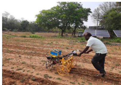
Figure 7.8: Solar power operated 3-tyne cultivator
