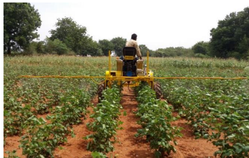
Figure 7.7: Spraying with tractor driven sprayer using high ground clearance platform Solar-cum-battery operated equipment
