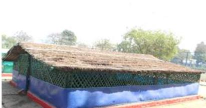
Fig. 1 Bamboo frame and thatched roof hut
