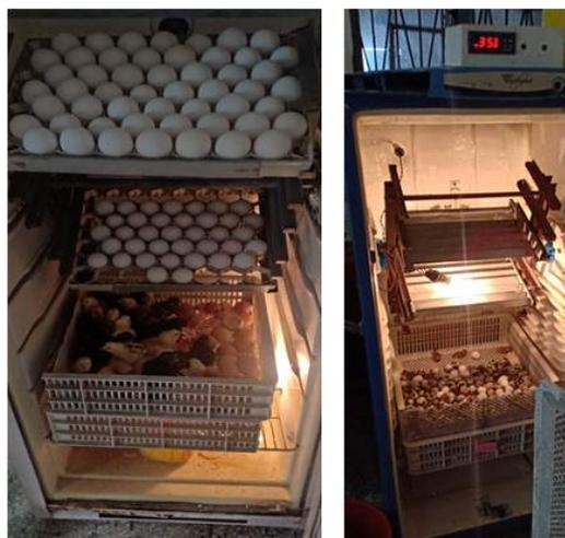
**Fig. 2. Front view of Rural poultry incubator fabricated from discarded refrigerator**
