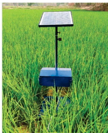
Fig.10. Eco-friendly Irrigation Alert System (e-IAS) in the paddy field
