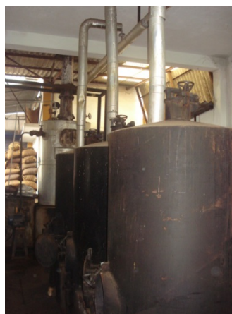
Fig 3. Steaming process for raw cashewnuts
